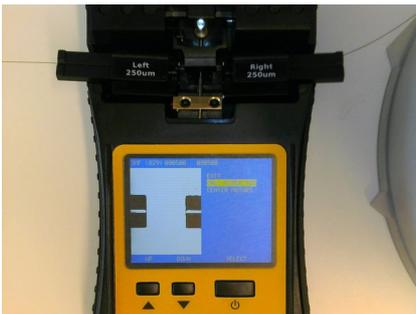
Check the fiber positions at top of the screen. They should be between 600 and 800.
