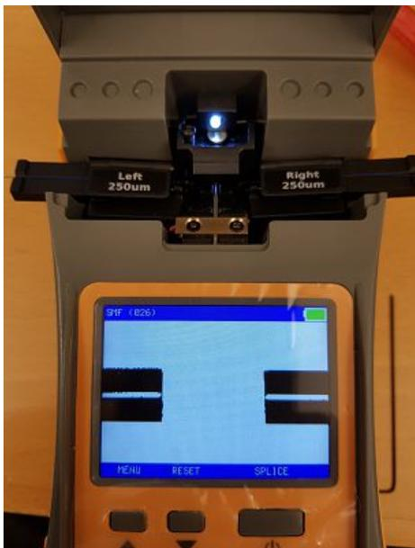
Put two fibers in place and check that they are positioned correct. If one is short and the other is long do a **FIBER POSITION** to set the correct fiber positions.
