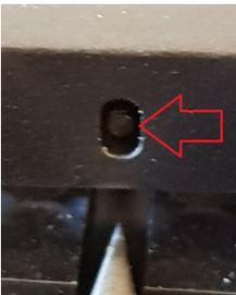
Verify that the ball-bearings clamp the fibers in the v-groove by lifting the fiber holder like in the picture below. Check that the fiber is moving horizontally but not vertically. Test both sides.
