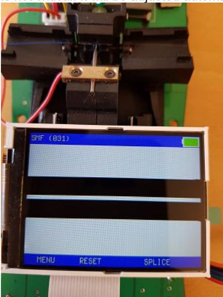
Turn off splicer and remove the camera-cable again. Tighten the screws a bit more so that the camera is secured but **don't over tighten the screws, the plastic threads might break**. Reconnect the cable and verify that the fiber is still perfectly horizontal.
