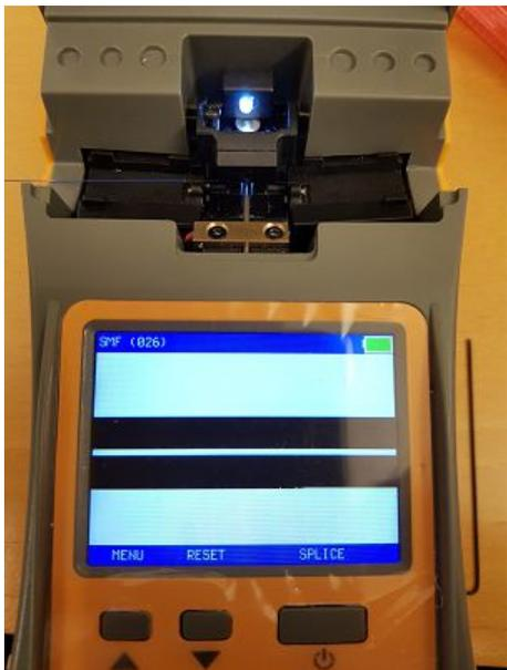
Put back the electrode and adjust it so that it is just outside of the screen. **Do not over tighten the screws,** just tighten to lock the electrode in place.
