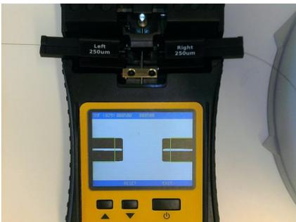
Two green boxes will be displayed showing the optimum position of the fibers.
