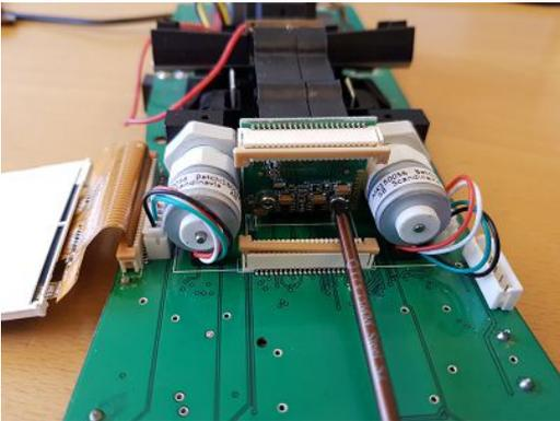
Now the camera is loose and You can clean the glass surface. Use wipes and fluids made for eye-glasses.
