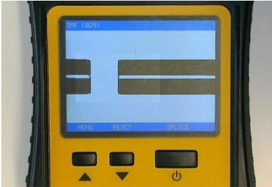
First thing to test is MENU/SETUP/FIBER POSITION/CAL. FIBER POS
