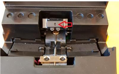
Insert fibers and adjust the height so that the ball bearing knob is in the center of the oval hole.
