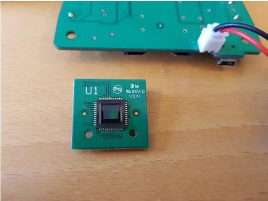
Put the camera PCB back in place. Tighten the screws so that it is still possible to move the camera. Connect the buttons and turn on the splicer. Put a fiber in the v-groove.
