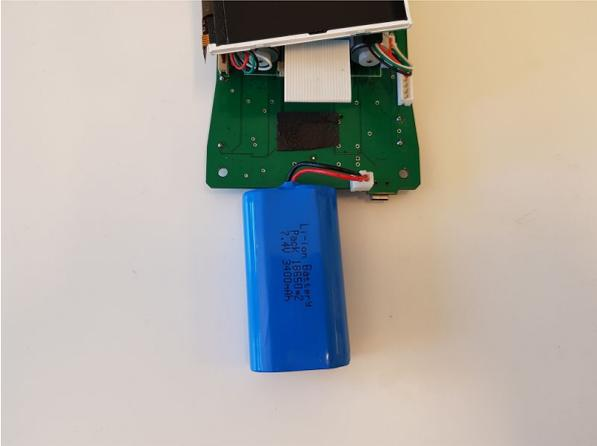
When putting the PCB back in place, make sure that the LCD display is in the correct place. You can look at the front side that it is in position. Also make sure that no cables have been placed where the screws will go to hold the bottom in place. Put back the bottom and the 6 screws.
