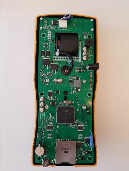
Now You can lift the PCB a little bit, enough to see the connector that should be disconnected.
