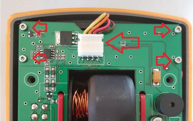
Now You can lift the PCB a little bit, enough to lift the old oven out.
