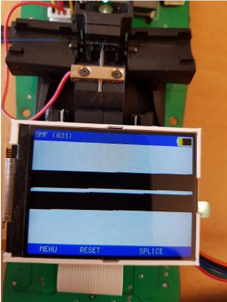
Rotate the camera until the fiber is perfectly horizontal like the picture below. The vertical position of the fiber is not critical. It will be adjusted automatically by the **CALIBRATE** below.
