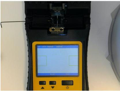
Remove the fiber-holder and adjust the small screw to adjust fiber length. Screwing it inwards will make the fiber longer. Adjust very little and test the new position by inserting the fiber-holder, fall down the clamp and press reset. Adjust until fiber fits into the green box.
