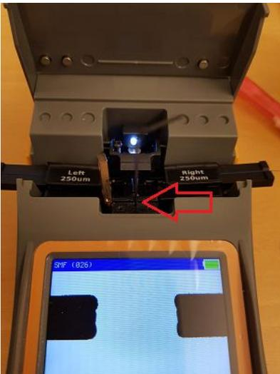
Use a 0.9mm Allen-key to loosen the lens. It is the screw closest to the white led (red arrow). **The screw closest to the screen is height adjustment for the electrode, don't adjust this screw.**
