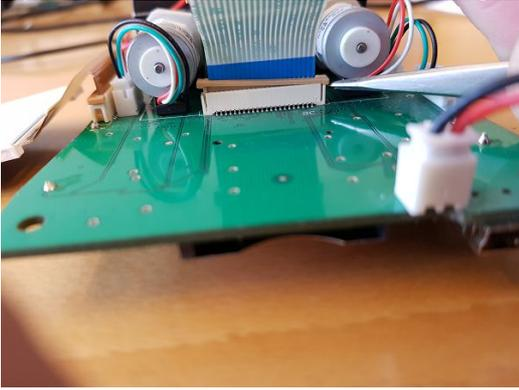
Remove the cable and the two screws that holds the camera PCB.
