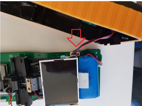
Now the battery can be removed. It is fastened with double sided tape so it may have to be cut away carefully.
