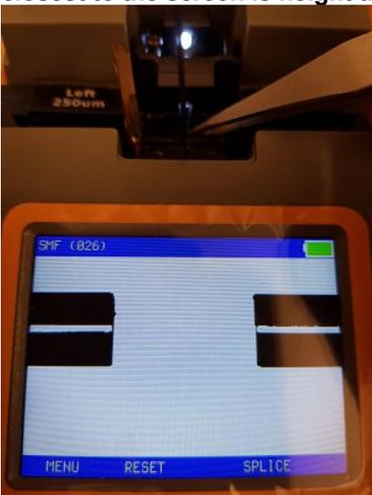
Adjust focus by moving the lens in or out (carefully, it is probably very loose). Lock with the screw when focus is good. Don't tighten very hard, just so that the lens can't be moved. **The lens tube is made of plastic so it can't be locked too hard or it will break.** When adjusting and locking the lens, fiber positions will move. Next step will take care of this.
